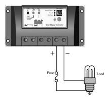
Figure 3-3 Load Wiring
