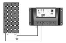
Figure 3-4 Solar wiring
