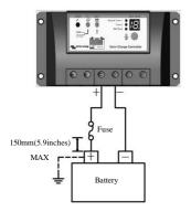
Figure 3-2 Battery connecting
