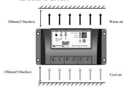
Figure 3-1 Mounting and cooling
